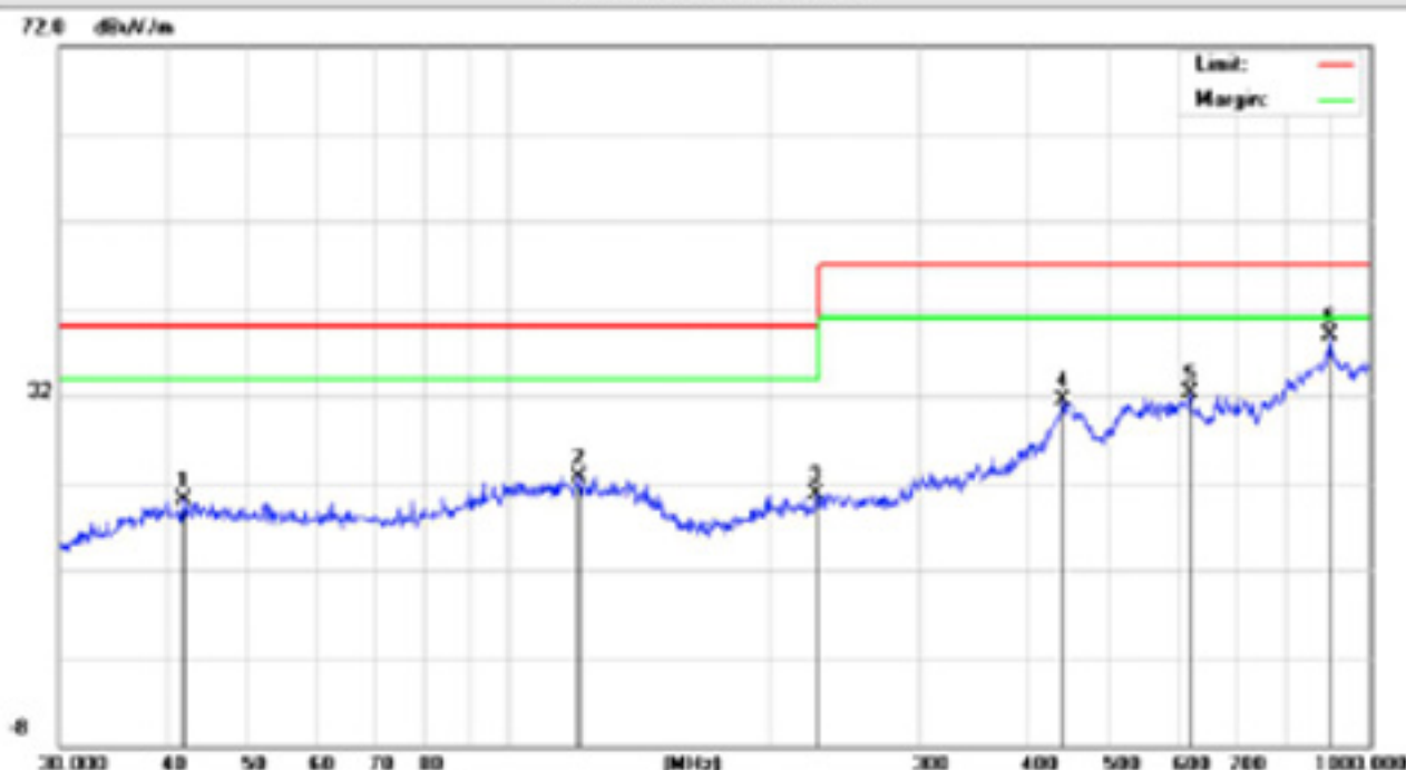
Test graph and data for Radiated Emission up to 1GHz Test Mode: Mode 1
